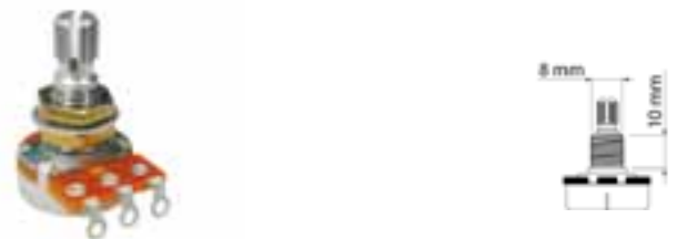
ALPS small 500K potentiometer, 16mm., 10mm. bushing, M8x0,75 thread, made in Japan
