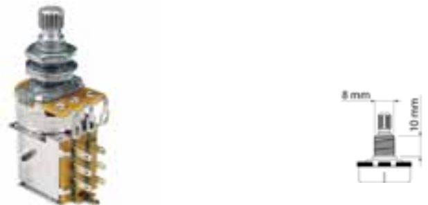
Ultra 500K push-pull potentiometer, 10mm. bushing, M8x0,75 thread, made in Korea
