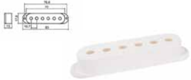
pickup cover, Stallion single coil, (small holes), 83,0-70,0x17,8x18,0mm, 5.2mm hole, 3 pcs
